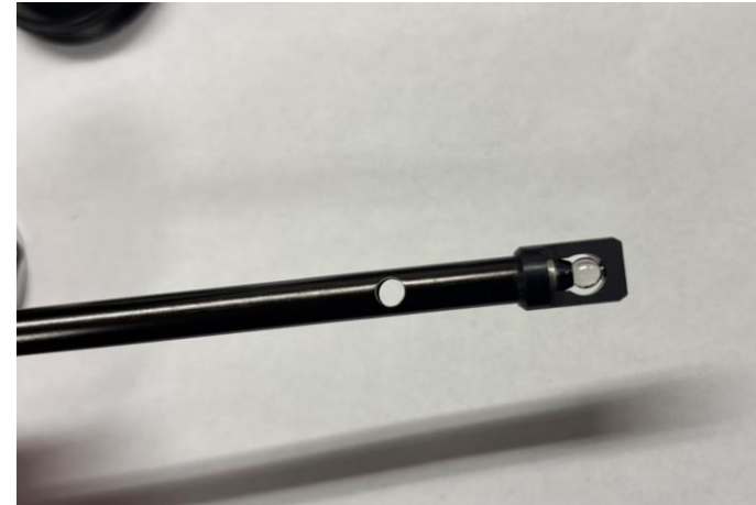
Glass ball reflector at the bottom of the pendulum
