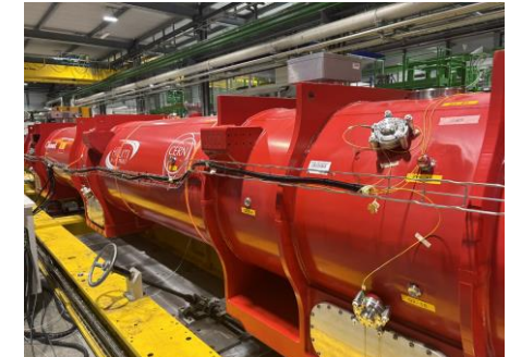
Low Beta quadrupole (on a test bench)
